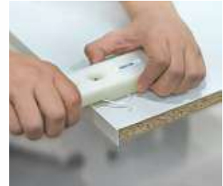
Clean trimming up to 3mm
