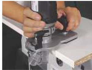
Easy trimming of either straight or shaped work pieces
